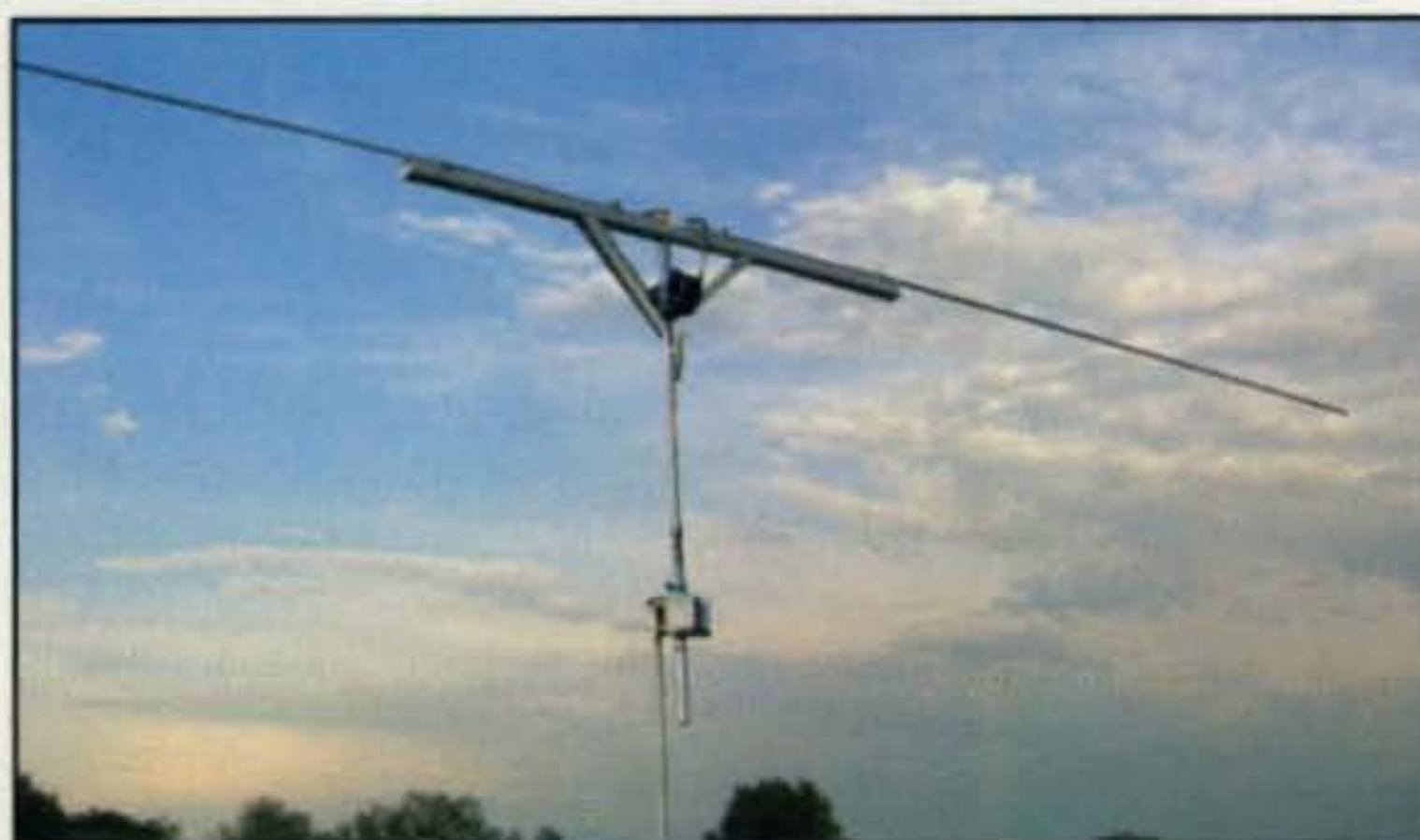
Photo A— W1XX's 17-meter adaptation of the classic "One-Element Rotary for 21 Mc." antenna designed by Lew McCoy, W1ICP, in the mid-1950s. The antenna was placed on a push-up mast and rotated with a TV-type rotator. Many QSOs resulted. (Photos by the author)
